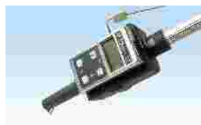
Fig. 4: Dose rate meter „X 5 C plus“ put on the Telescope adapter
