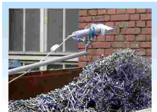
Fig. 1: Telescope adapter with NaJ-scintillation probe 2002 for controlling steel scrap with regard to radioactive contamination
